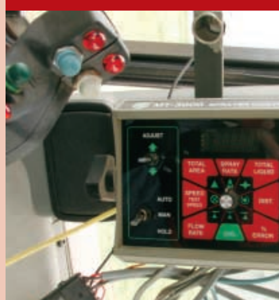
Spray Controller mounted inside the Ellington's tractor for use in conjunction with the global positioning technology.
